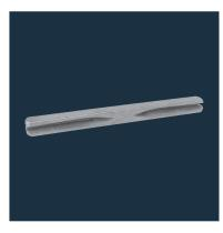
Spreaded spindle (8 mm) The fixing is carried out by a "set screw-headless with cone point" (DIN 914). The cone point enters the slot of the spreaded spindle. The spindle is pushed apart. Positioning necessary! Further lengths on request.
