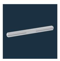
**Grooved spindle (8 mm)** For a high-strength connection (spindle / lever) for door handles. The fixing is carried out by a "set screw-headless with punch". Here the punch cuts into the groove. Positioning necessary!
